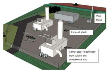
Figure 6: Compressor station overview (without a catalyst fitted)
