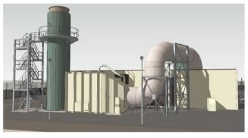
Figure 7: Compressor cab with SCR fitted
