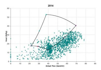
Based on the required duty, there would have been circa 600 and 1075 hours of operation that could not have been met at Hatton without additional compression in 2010 and 2014 respectively. The analysis excludes operating points associated with compressor start up. Given the combination of the normal operating duty being well in excess of 500 hours and the potential constraint costs, we conclude that the cost / benefit of installing one new unit is robust.
