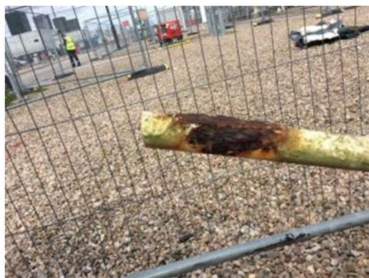
Figure 9: Through wall corrosion requiring replacement to continue operation
