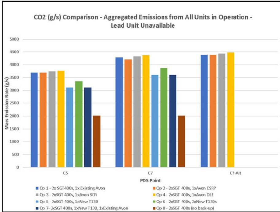
Figure 8-7: Comparison of Aggregated CO Emissions – Lead Unit Unavailable
