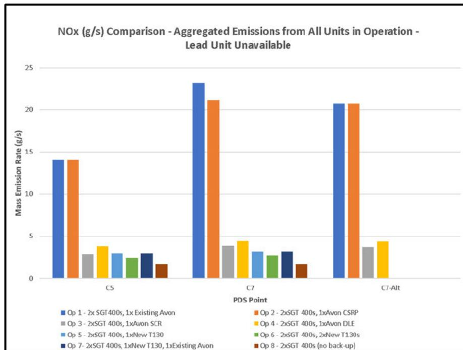
It is evident from the data presented above that there are differences in the CO<sub>2</sub>, CO and NOx emission rates calculated for each PDS point across the operational scenarios assessed. However, the patterns identified above are not consistent across each option and pollutant, and rather than reviewing the mass emission rates in isolation, the data should be considered alongside the operational hours of each individual unit across all PDS points.
