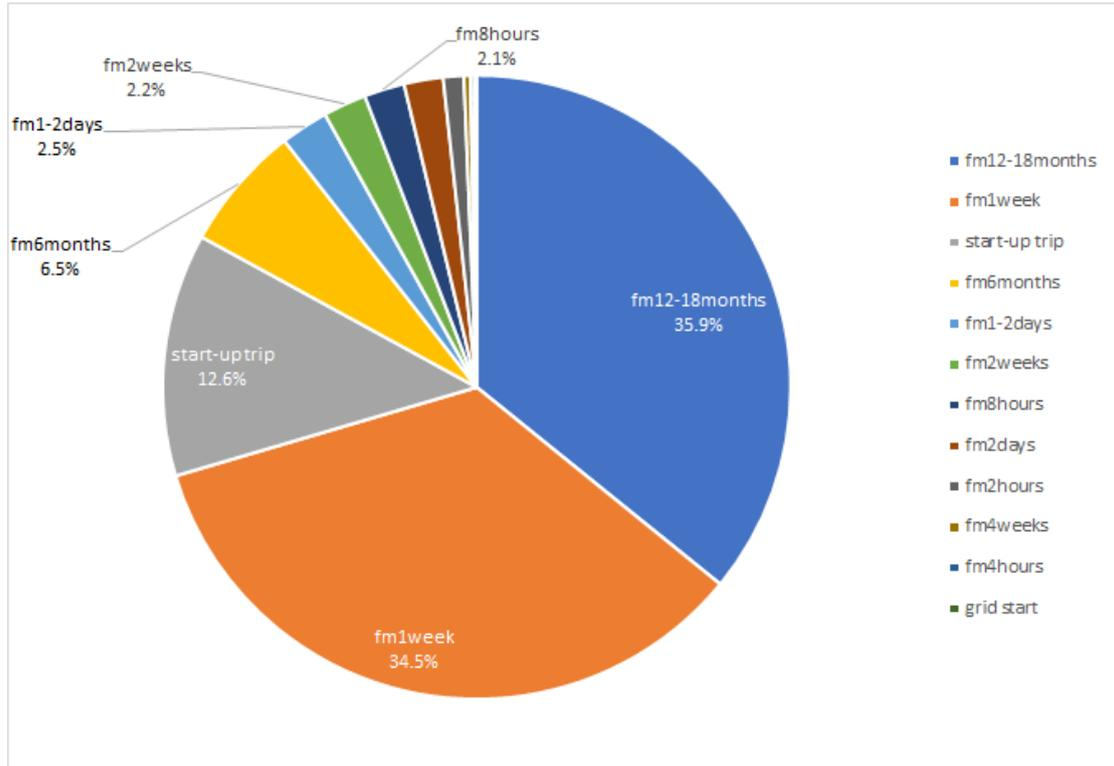
**Figure 3-9, VSD – Failure Mode Contributors**
