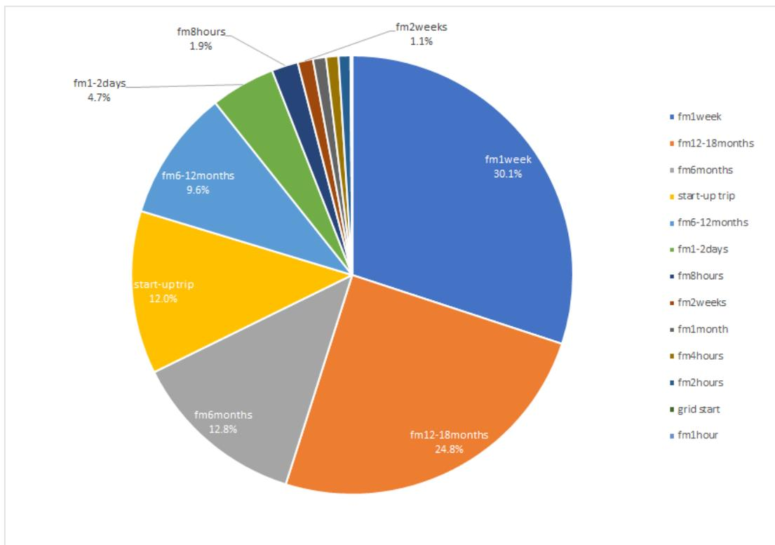
Figure 3-3, Avon – Failure Mode/Repair Time Contributors
