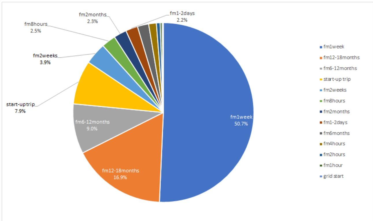
**Figure 3-6, SGT400 – Failure Mode/Repair Time Contributors**
