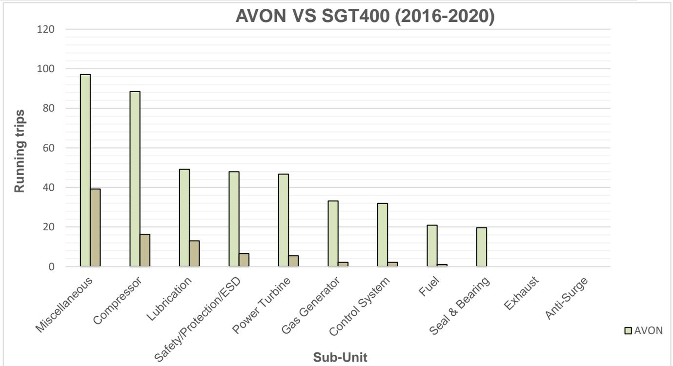
**Appendix A - 12: Bar chart of sub-unit running trips for Avon vs SGT400 units (2016-2020)**
