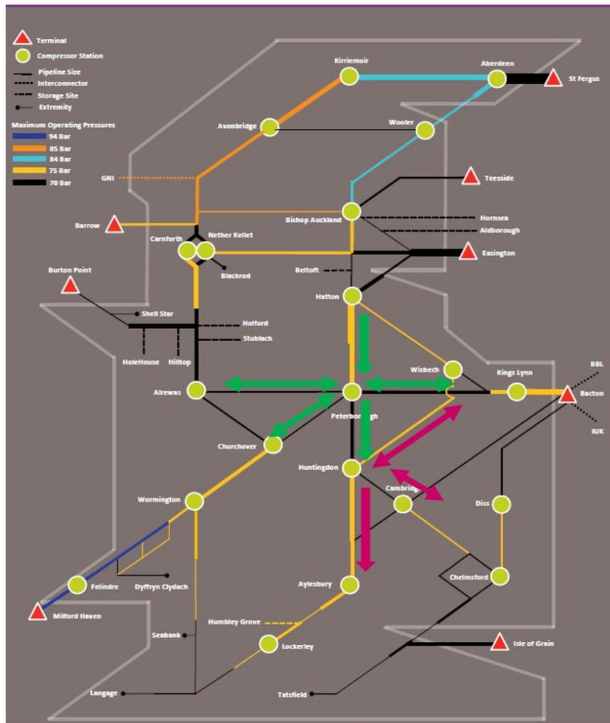
**Figure 9** - Schematic of the National Transmission System (NTS) indicating potential multi-junction configurations for Peterborough and Huntingdon compression
