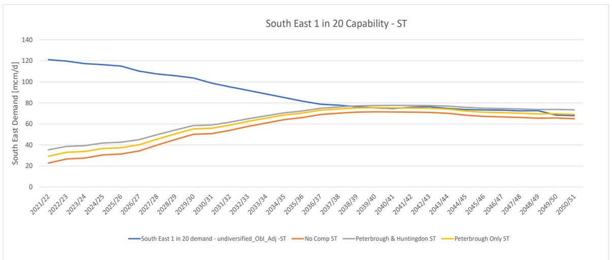
**Figure 14 - South-East 1-in-20 demand forecast along with network capability provision for the ST scenario for various compressor options**
