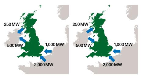
*Figure 2.7 Projected interconnector flows for peak and off-peak times for summer 2017*
