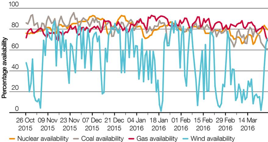
To understand the availability of different generation types in more detail, figure 4 shows the availability of nuclear, coal and gas for the peak periods of each day across winter 2015/16. As wind has a significant impact on how our forecast compares with actual generation, wind availability has also been included. The total availability includes both planned outages and breakdowns.
