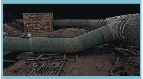
3D As Built – an example section of the laser-scanned pipework that will provide improved knowledge on the pipework after burial.
